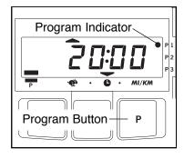
the manual mode, press the program button until the program indicator disappears. The programs will be selected in the following order: program 1 (Interval), program 2 (Aerobic), program 3 (Fat Burn), manual mode.
